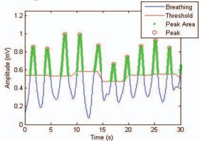
Figure 3. Breathing Peak Detection. The breathing signal (solid blue line) is filtered using the dynamic threshold (solid red line) to find the discontinued peak areas (green asterisks). The threshold is calculated by adding 10% to each mean value determined over 5sec non-overlapping sliding windows. Finding the time of the local maximum in each discontinuous peak area determines the peak times (red circle).
