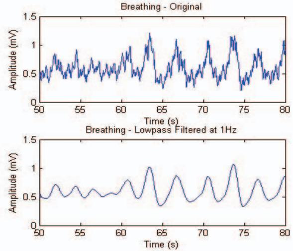
Figure 2. Filtering of Breathing Signal while Running. The top plot shows the raw breathing signal from the breath sensor during a run. Notice the noise caused by body movement making it difficult to discern low amplitude breathing signals. Lowpass filtering at 1Hz shown in the bottom plot effectively removes the unwanted signals.
