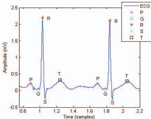
Figure 4: PQST Peak Detection is performed after initial R-Peak detection. With known R-Peaks, we find the preceding and following local minima to obtain Q and S, respectively. P can then be found by finding the local maximum preceding Q. T is found by finding the local maximum following S. Time windows are used to determine the local max/min. The size of the time windows is dependent on the period between R-Peaks.
